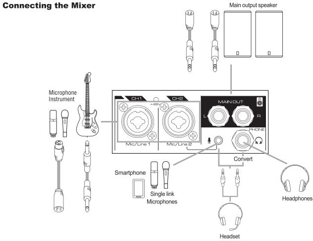
Astatic M2 is a multipurpose 2 channel (2mic/line) analog mixer with a built-in USB interface. USB connectivity and +48V phantom power make it an ideal compact option for live performance, broadcasting, podcasting or home recording.
