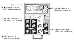
Note: if a condenser microphone is used, please turn on the switch of ( ) 48V phantom power supply.
